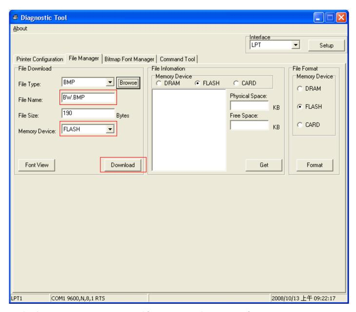
3. After file downloading, enter the tab [*Command Tool*] and edit a TSPL2 program to print the BMP graphic on label.
